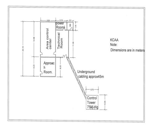
Figure 1 Layout of JKIA ACC, Approach, Equipment and Control Tower Rooms at JKIA
